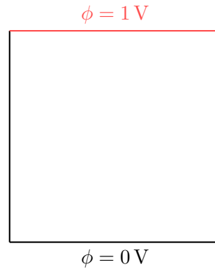
Figure 1: Electrostatic problem in vacuum to solve. An empty space is delimited by 4 conductors. Three of them (in black) are at zero potential, the last one (in pink) is at a potential of 1 volt.
